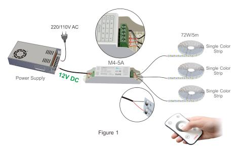
E.g. 2: Connected 24V lamp, loads1~480W(24V).
